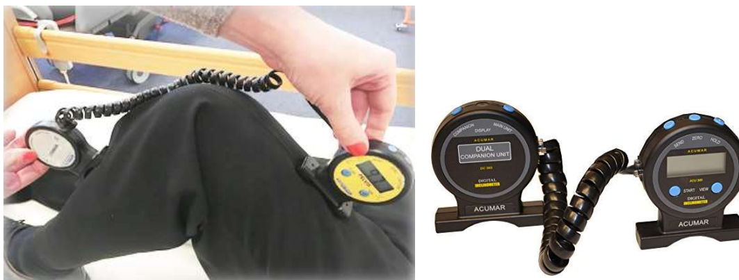
Acumar™ Dual Digital Inclinometer in use with model.
