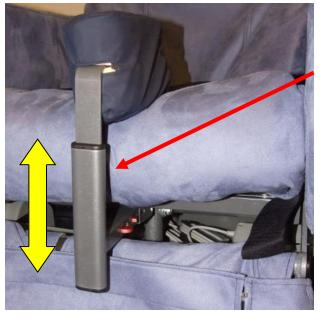
Should it be necessary to change the pommel head size or adjust the height of the pommel first locate the screw behind the stem.
