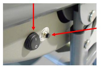
To protect the unit from damage there is also a reset/trip switch fitted. If the unit stops working, firstly check the power switch is on.
