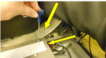
To set the seat depth, first remove the seat cushion and locate the two locking screws at the back of the seat plate.
