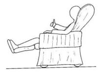
The user must always be positioned within the wheel base of the chair. A posture belt may be necessary to achieve this at all times.
