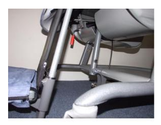
It may be necessary to adjust the angle of the footplate to get the user's foot fully supported. The lever to adjust the footplate is underneath the plate and is show in red below.
