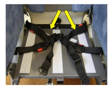
Remove the seat cushion and locate the rear and side seat mountings.
