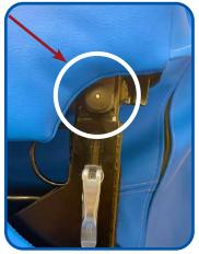
Located towards the back of each arm on the outside - as shown, is a small release knob that needs to be pulled out whilst lifting the arm up.
