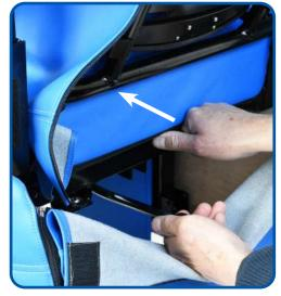
Remove the lower, rear zipped cover to reveal the adjustment lever and handle on back of seat pad. Gently pull the lever upwards and at the same time **PUSH** the cushion handle/pad away from you to correct/desired position.
