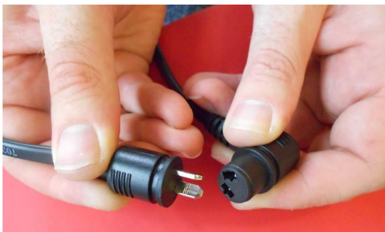
RE-CONNECTING THE CHARGER CABLES
